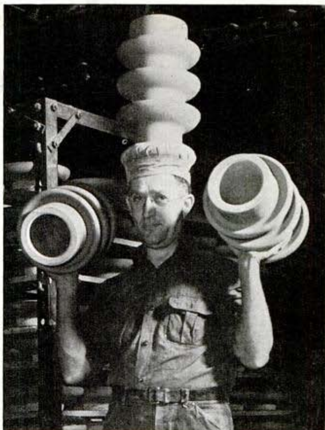
Carrying a 20-pound insulator on head helps speed production
